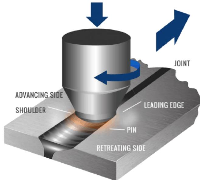
Figure 8: Friction stir welding
