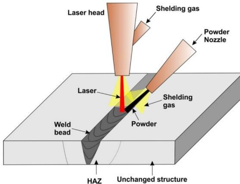
Figure 10: Laser welding
