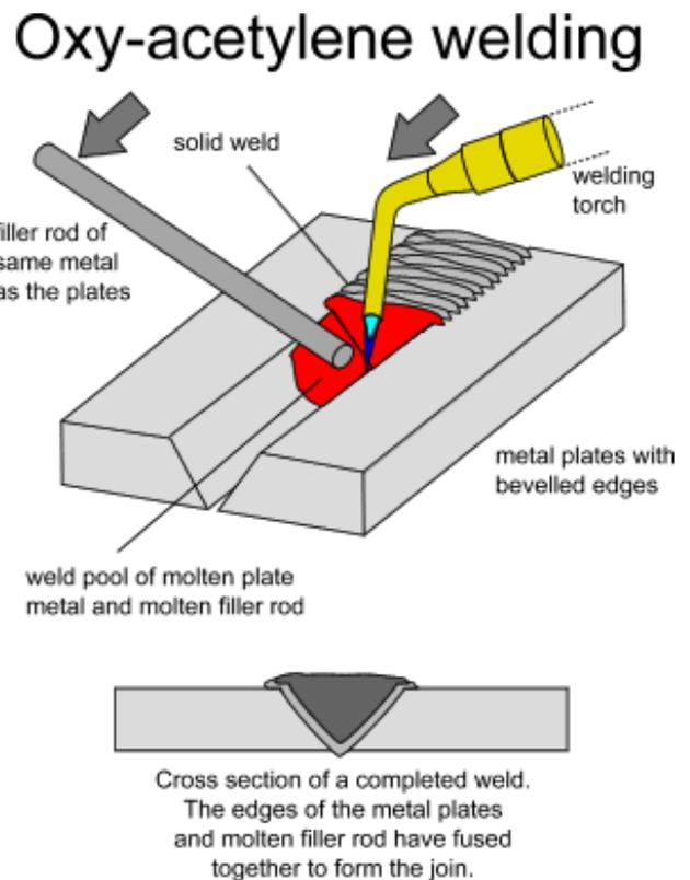
Figure 7: Oxy-acetylene welding
