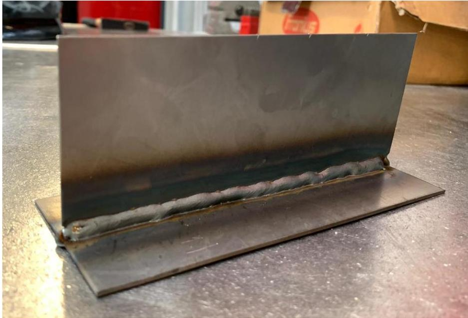
Figure 41: T-Joint weld
