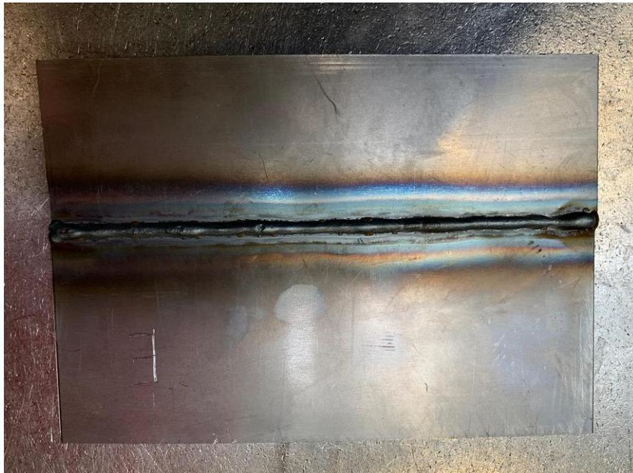
Figure 42: Butt weld
