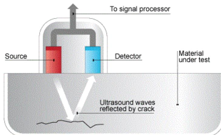
Figure 16: Ultrasonic Testing
