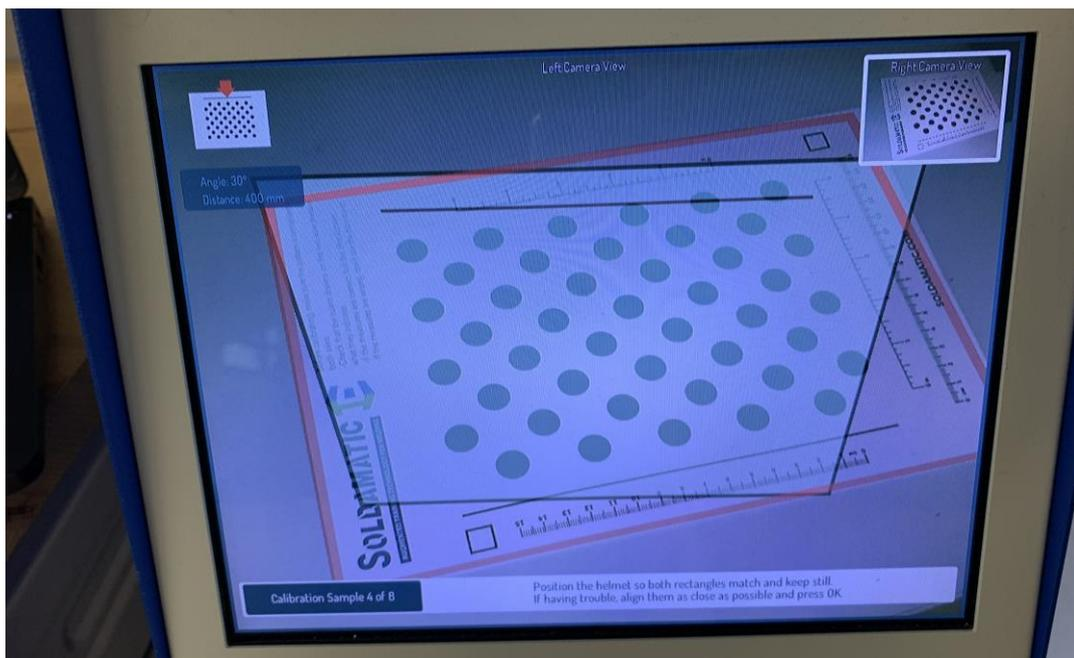
Figure 19: Calibrating of SOLDAMATIC
