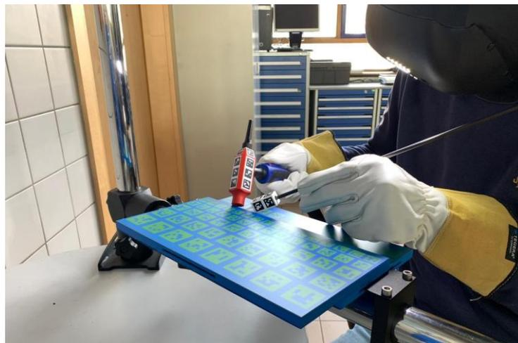
Figure 32: Augmented Reality Welding
