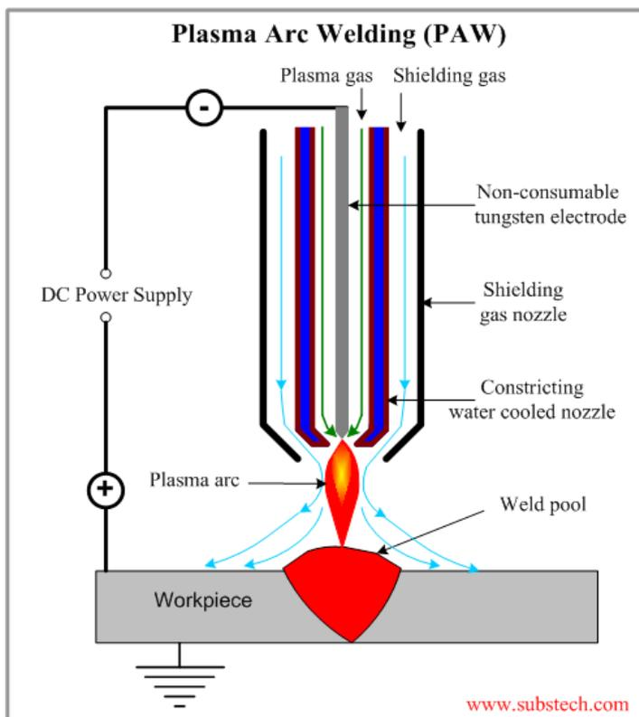
Figure 6: Plasma arc welding
