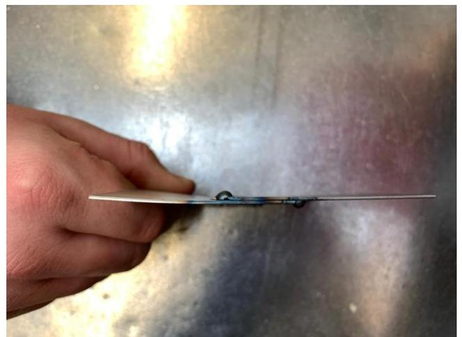
Figure 40: Overlap welding side view
