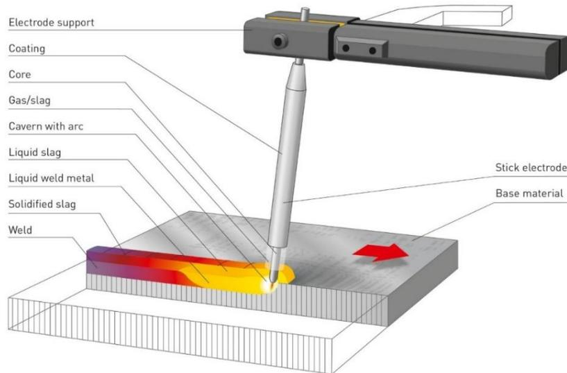
Figure 4: Arc welding
