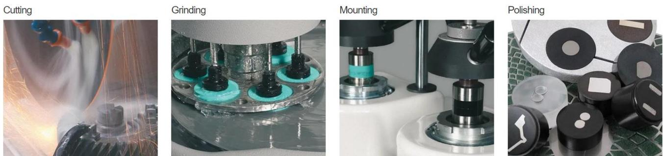
Figure 15: Metallography Examination stages
