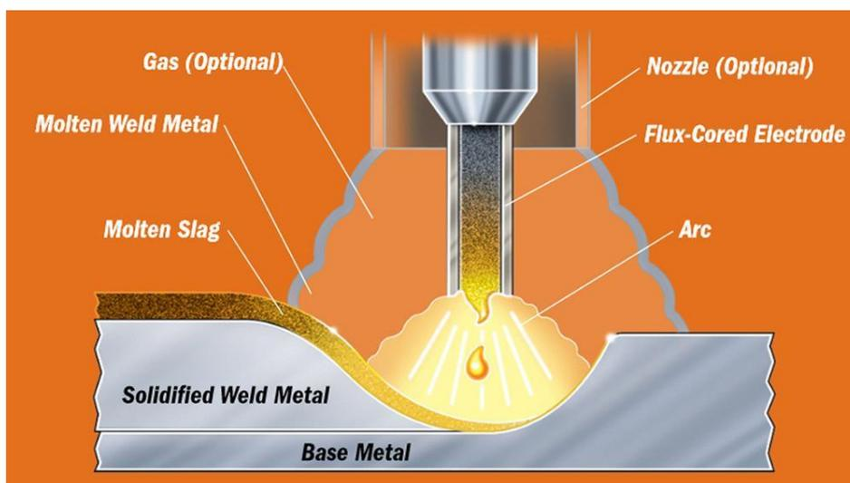
Figure 5: Flux welding
