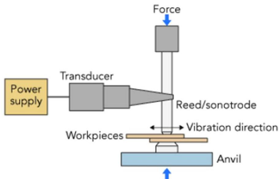
Figure 9: Ultrasonic welding
