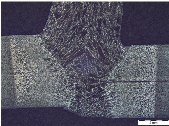
Figure 49: HAZ on Butt weld
