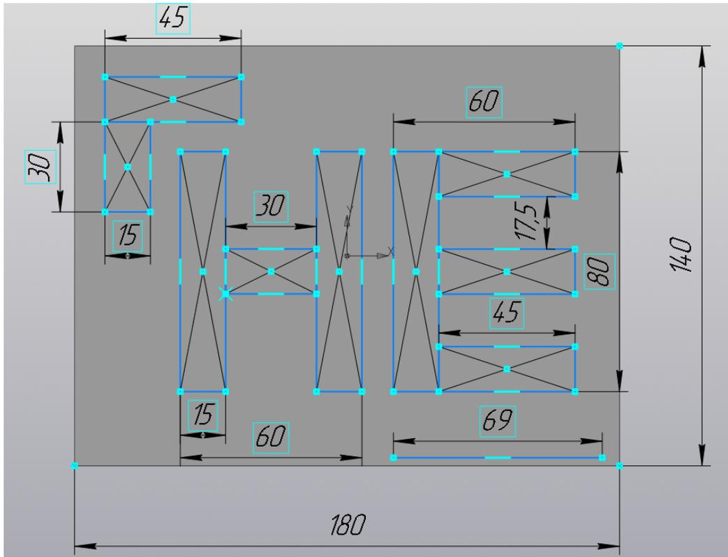
Figure 30: Dimensions of the HS plate
