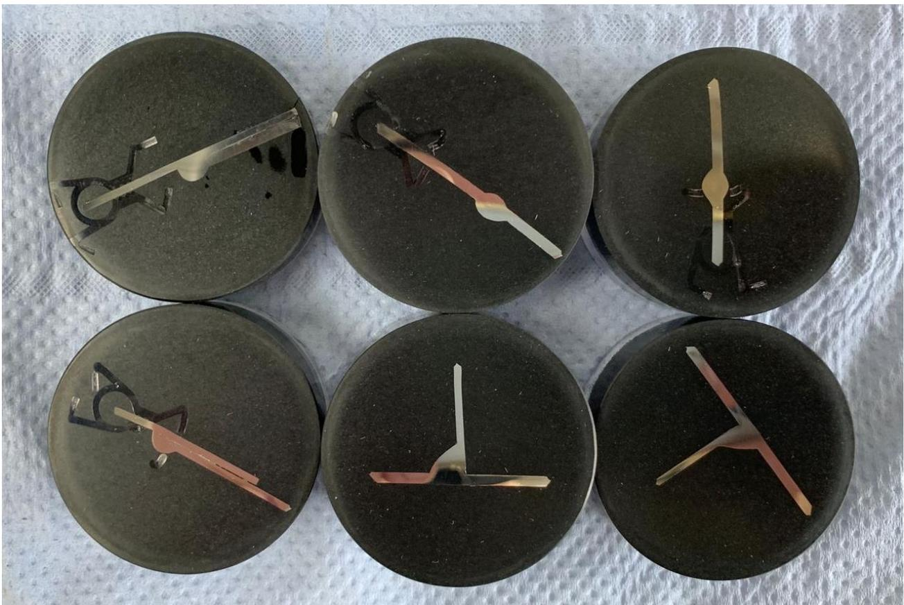
Figure 48: Specimens for Microscopy
